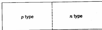
Figure 24 A p-n junction is made from a single crystal modified in two separate regions. Acceptor impurity atoms are incorporated into one part to produce the p region in which the majority carriers are holes. Donor impurity atoms in the other part produce the n region in which the majority carriers are electrons. The interface region may be less than 10^{-4} cm thick.
