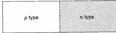
Figure 24 A p-n junction is made from a single crystal modified in two separate regions. Acceptor impurity atoms are incorporated into one part to produce the p region in which the majority carriers are holes. Donor impurity atoms in the other part produce the n region in which the majority carriers are electrons. The interface region may be less than 10^{-4} cm thick.
